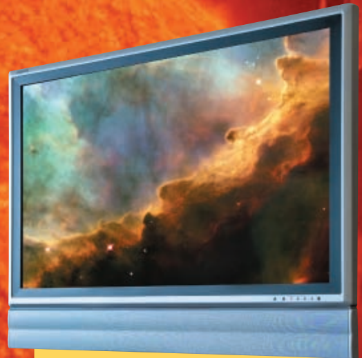
A high voltage in a noble gas, such as neon or xenon, produces the plasma in displays like this.
